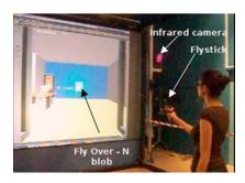
Figure 4. Experimental setting with the use of Fly Over on the semi-immersive platform. Users navigate by moving a Flystick in their hand, which position is computed by two infrared cameras.
