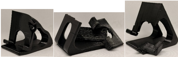
Figure 10. Smartphone holder models after experimental testing.
