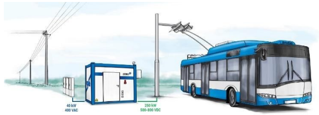
Fig. 6. Fast charging station with storage energy system designed by AREX company (Gdynia) – CAR project
