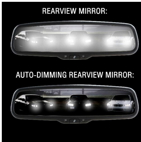
Fig. 4. Difference in glare between a classic (prismatic) and electrochromic rear-view mirror
