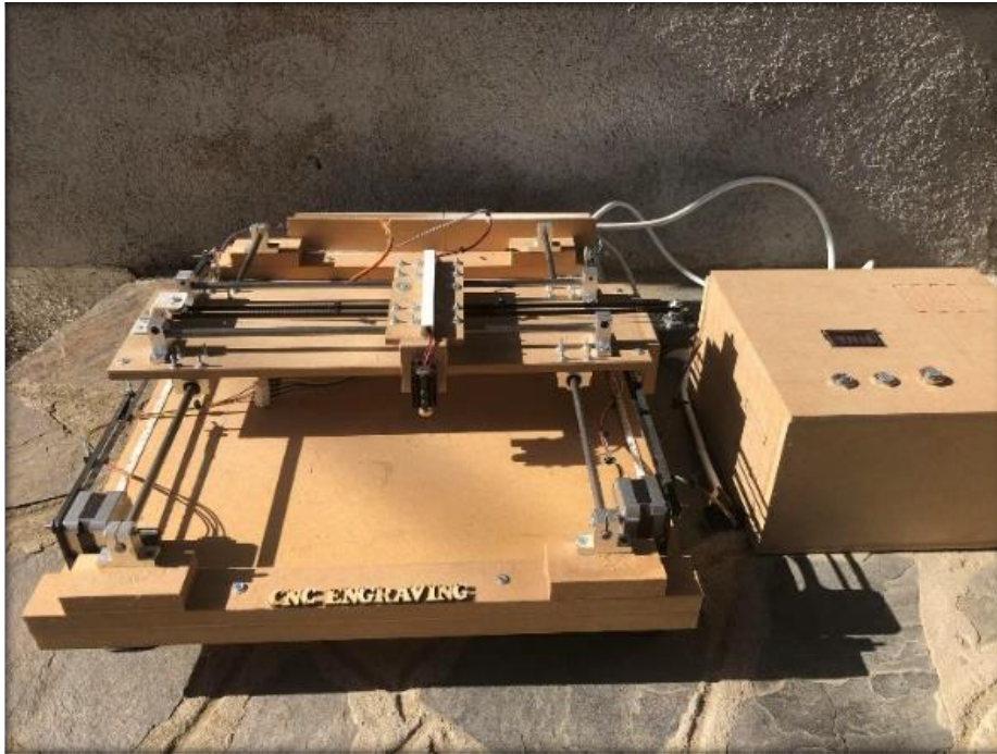
Figure 2: Hardware model of CNC laser engraver
