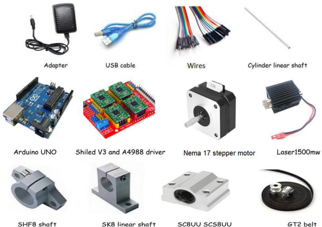
Figure 1: Component of the Laser engraving machine
