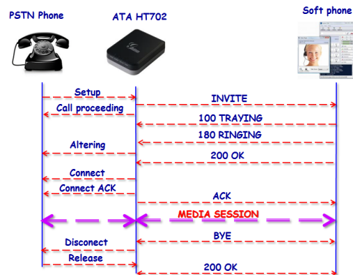
Fig. 5. Establishing a call to the known IP address between the analog phones integrated with the ATA H702 in the VoIP system.
