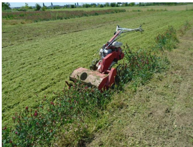
Photo 1. Gasoline-powered mini-tractor Honda F-620 Y coupled with MIO Standard mulcher used to chop the crimson clover herbage in previous researches
