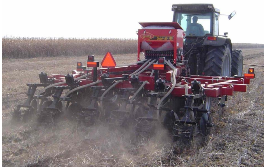
Figure 1. Strip till equipment Case DMI 5310 with dry fertilizer box
