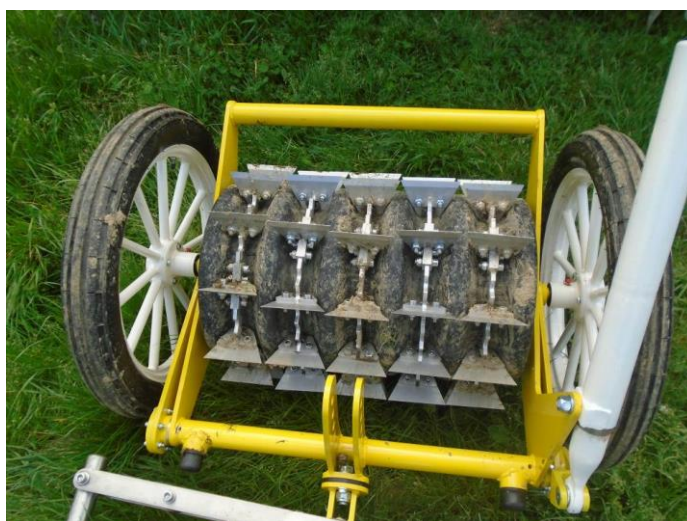
Photo 2. Blades on steel rings over the rubber drum on horse-powered roller-cutter for chopping the crimson clover herbage in this research (designed by Schaff mat Paerd asbl., Luxembourg)
