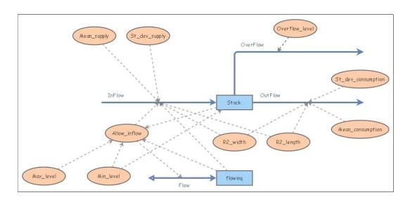
Figure 1. Water tank "R2", as modeled in Insight Maker®
