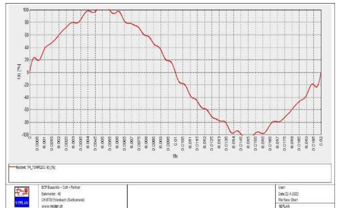
Figure 7 Current of the transformer TR_TORPEDO (2x500 kW) with filter of 3 rd harmonic
