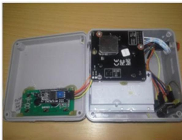
Fig 1. PM IoT node prototype
