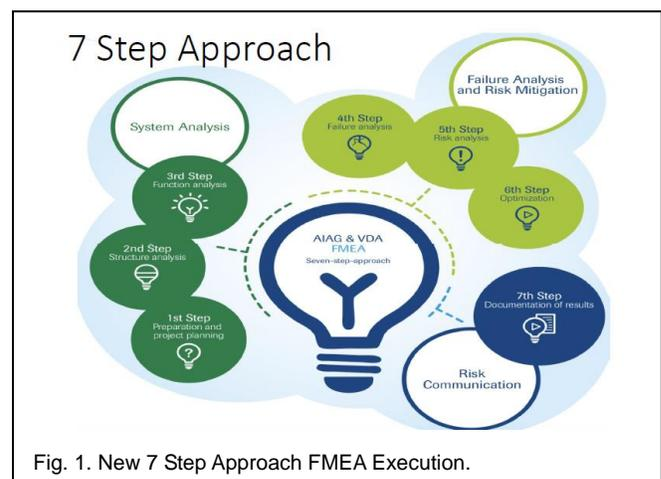
Fig. 1. New 7 Step Approach FMEA Execution.
