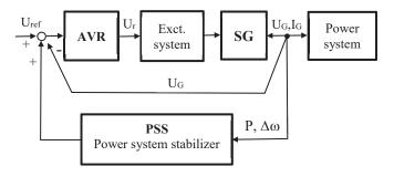
Fig. 2.1 Conventional structure of the system for managing the excitement of the synchronous generator
