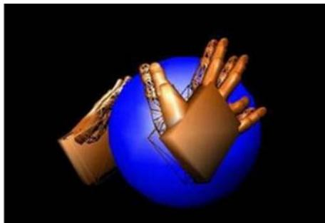
**Figure 5. Holding a Ball with Two Virtual Hands; the Opaque Hands Show the Positions of the Virtual Hands, the Wireframe Hands Show the Positions of the User's Real Hands. They are, in contrast to the virtual hands, able to penetrate the ball.**
