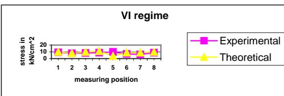
Fig. 8 Strain of clamps at measuring positions under dynamic loads in Sixth working regime of the excavator
