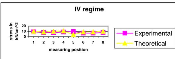
Fig. 6. Strain of clamps at measuring positions under dynamic loads in Fourth working regime of the excavator
