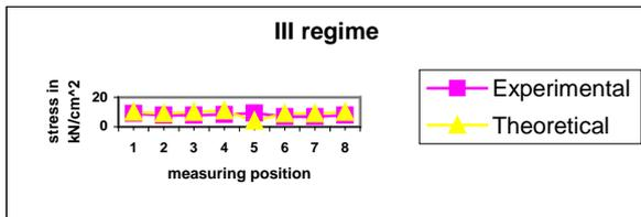
Fig. 5 Strain of clamps at measuring positions under dynamic loads in Third working regime of the excavator
