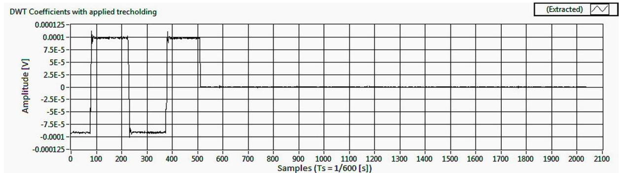
Fig. 8. Detail coefficients processing for denoising purposes .
